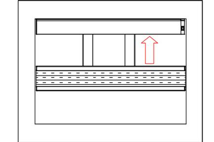
\* When middle rail & bottom rail meet the head rail, it is top limit.
