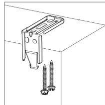
Use two 1 1/4" installation screws to secure brackets. Use wall anchors for drywall or plaster wall.
