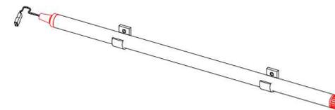
Please remove the clips from the batter wand before you install the clips.
